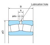
Lubrication holes and groove
