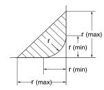
Remark: The exact shape of the chamfer is not specified, but its contour will be in the area shown with oblique lines.
