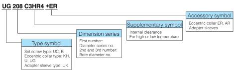
Note: For type B bearings, a last digit of bore diameter number is used as dimension series number.
